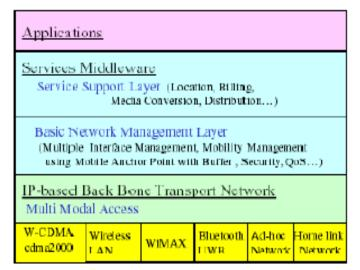
Fig. 2. View of the IP-based 4G mobile and wireless network architecture.
